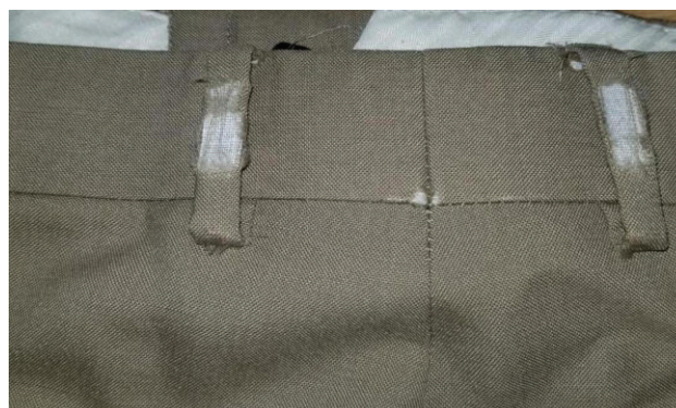
The rear waistband and belt loops of these slacks are beginning to rip from repeated abrasion in use.
